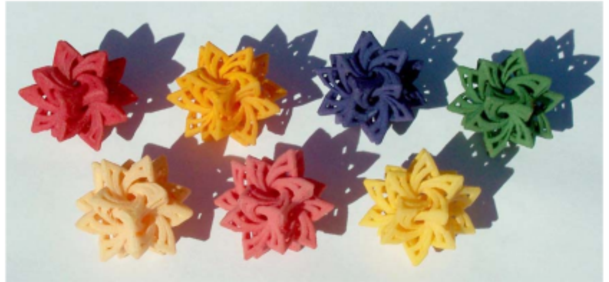
Frabjous gift exchange: 1 inch nylon models, of selective laser sintering, colored.
